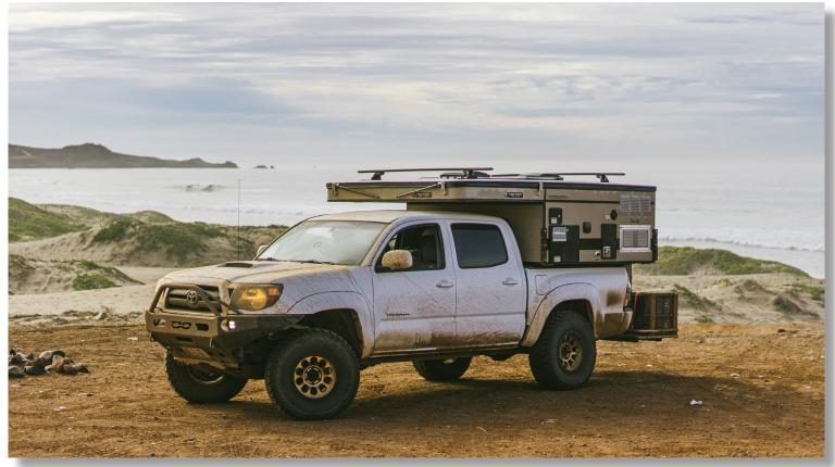
Dry Weight: 935 Lbs. Adult Sleeping: 2-3 Height Down (including vent): 54" Extended Interior Height: 6'4" Roof Length: 111" Roof/Wall Framing: Aluminum Floor Length: 70" Exterior Material: Aluminum Body Width: 75"
