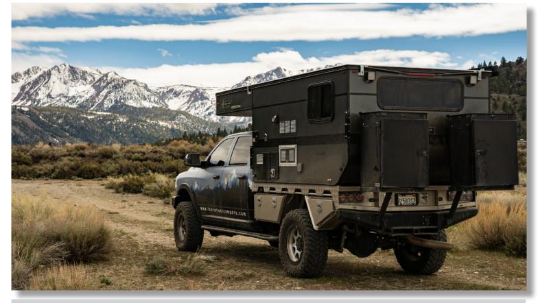
Dry Weight: 1,395 Lbs. Adult Sleeping: 3-4 Height Down (including vent): 60" Extended Interior Height: 6'6" Roof Length: 165" Roof/Wall Framing: Aluminum Floor Length: 94" Exterior Material: Aluminum Body Width: 81" Fresh Water Capacity: 20 Gallons
